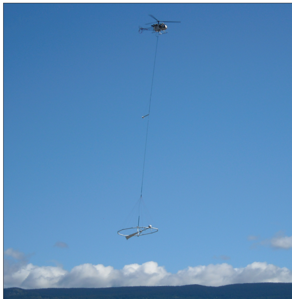
Aerial insight: Aeroquest’s airborne electromagnetic system collects data using a large loop suspended beneath a helicopter that flies at low altitude
